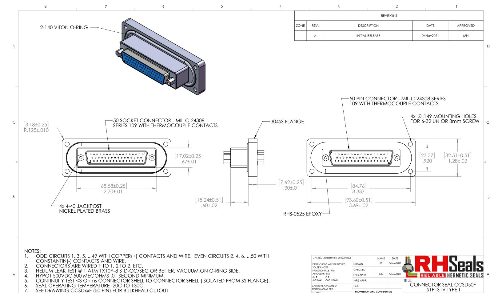
DIMENSIONS ARE INCHES [MILLIMETERS], MILLIMETERS SHOWN FOR REFERENCE ONLY.
